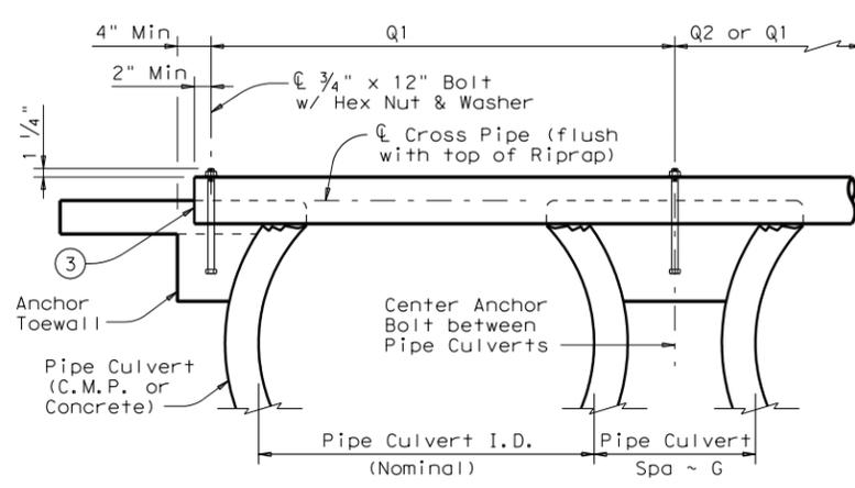
**SHOWING CROSS PIPE WITH BOLTED ANCHOR**
