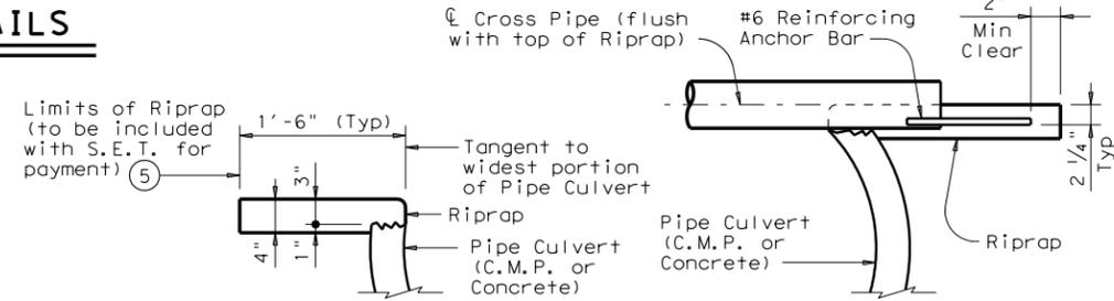
**SHOWING TYPICAL PIPE CULVERT & RIPRAP**
