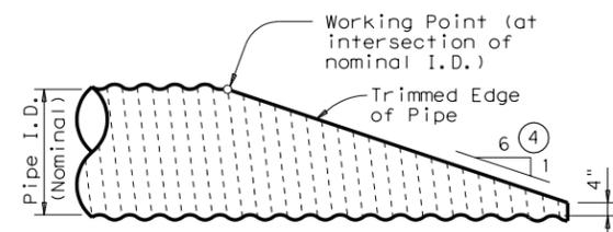
NOTE: All Cross Pipes, calculations, and dimensions are based on the pipe culverts mitered as shown in this detail. Alternate styles of mitered ends will require that appropriate adjustments be made to the values presented on this standard.
