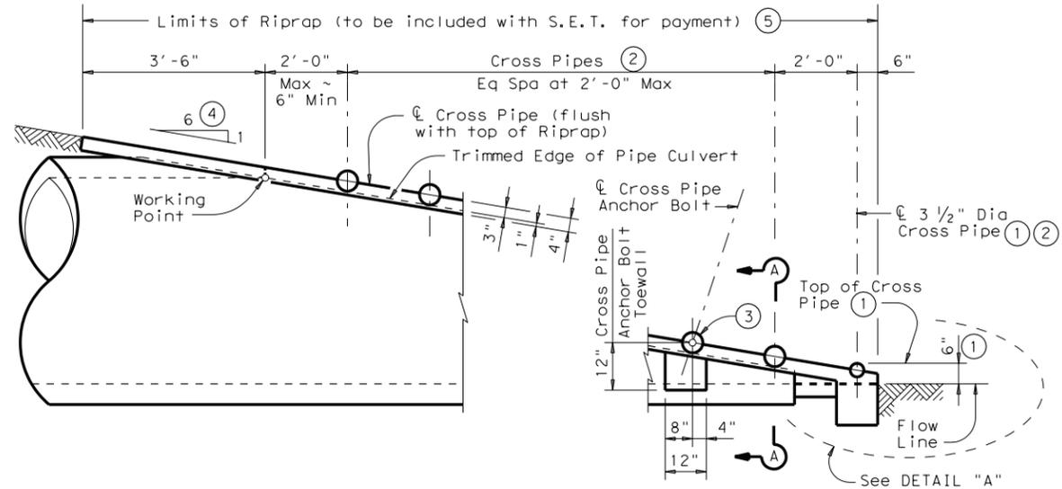
**SIDE ELEVATION OF CAST-IN-PLACE CONCRETE**
