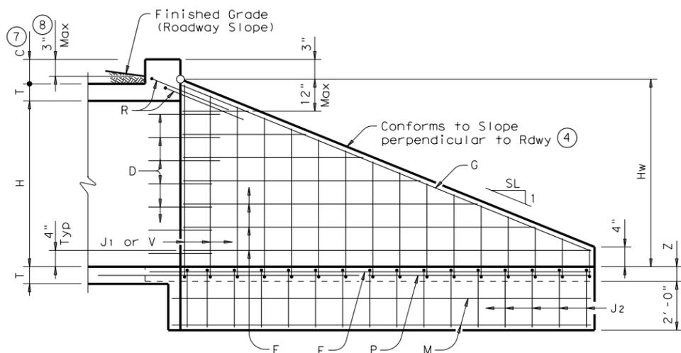
Length of Wings based on SL:1 slope along this line.
